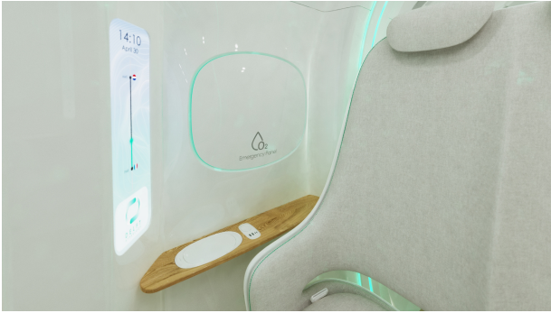
(a) Passenger seat inside the hyperloop pod as designed by Delft Hyperloop V. The seat is provided with a screen for information about the itinerary, and contact with the hyperloop operator, when necessary. On the side of the chair an emergency kit is located, to be used in case of a pressure drop inside the cabin.
